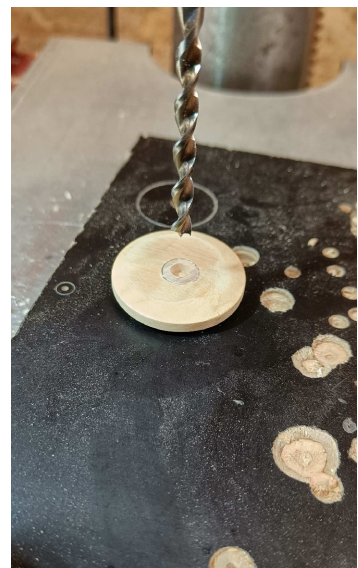
Drilling a 5mm hole on the backside
